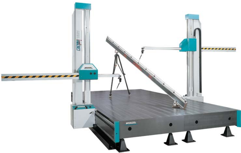
Figure 1: KOBA-Ball Bar on a CMM of horizontal arm type
